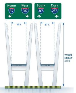
transverse tower strut – a structural element typical between two towers – adding to the open air experience while crossing the bridge. This solution achieves a clean aesthetic, has vastly improved safety features and provides a high-quality, low-maintenance replacement for this critical crossing.
